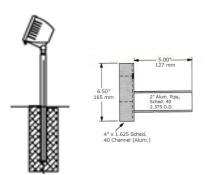
The FB fixture bracket is a small aluminum pipe that is direct buried into the ground to mount the fixture. The ST side of pole tenon bracket is a straight arm ranging from 5" to 24" to provide a close to pole mounting option. The HB is a small arm for installations on the side of a flag pole or out in front of a sign.
