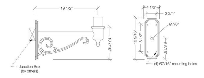
The London Bracket (LB) is used for mounting the London decorative fixture to the side of the pole below the solar power assembly. This decorative cast aluminum scroll bracket is 16" and comes ready to mount to the pole with the pendant style fixture above. Powder coated allows for customization of the bracket to match the color of the pole and fixture.
