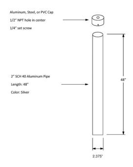
The Fixture Bracket (FB) supports ground mounted flood lights, uplights, flag lights and landscape lights. The aluminum, steel, or PVC top cap comes with a 1/2" NPT hole in the center with a 1/4" set screw. The 48" x 2" Schedule 40 Aluminum pipe comes standard in silver but can be powder coated upon request.
