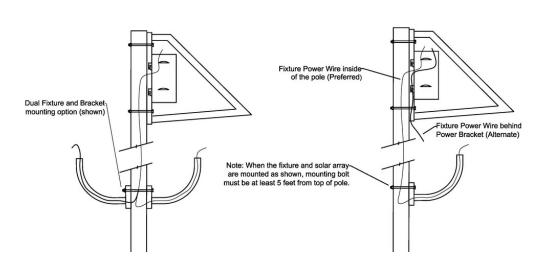
The Side of Pole Horn Bracket (SH) is a short 10" upsweep bracket used to mount a flood fixture on a pole or wall. The wire can be routed inside the pole and into the back of the bracket foot for no exposed wiring. Brackets are standard in brushed aluminum but can be powder coated to match the fixture color.
