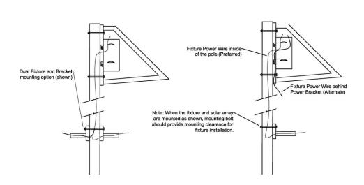
The Side of Pole Tenon Bracket (ST) is a short straight bracket arm for close to pole installations. The bracket is available in 5" and 24" lengths. The wire can be routed inside the pole and into the back of the bracket foot for no exposed wiring. Brackets are standard in brushed aluminum but can be powder coated to match the fixture color.
