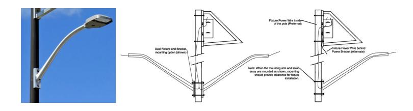
The Side of Pole Bracket (SP) is an elliptical aluminum bracket available in a 4', 6' and 8' length standard with a 2' upsweep, longer lengths are available upon request and specification requirements. The wire can be routed inside the pole and into the back of the bracket foot for no exposed wiring. Brackets are standard in brushed aluminum but can be powder coated to match the fixture color.
